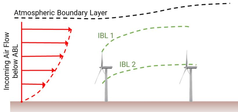
**Figure 3-8: Internal Boundary layer development**
