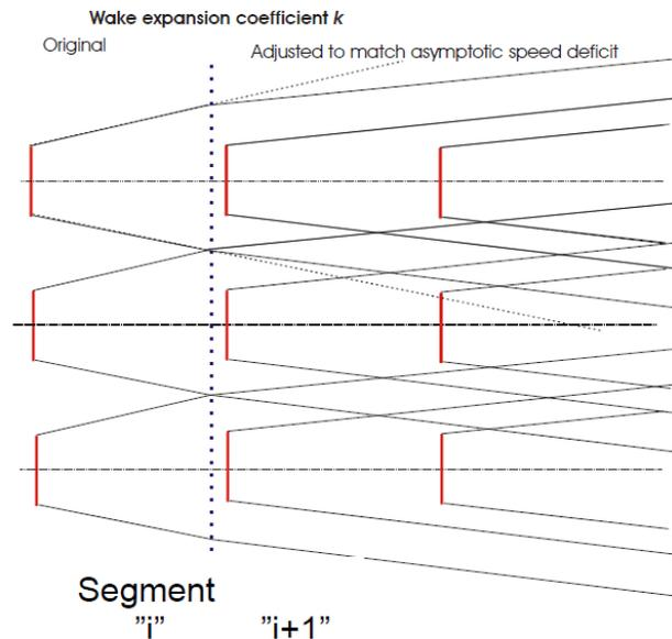
**Figure 3-7: Adjustment of wake expansion rate at downward wind turbines<sup>16</sup>**
