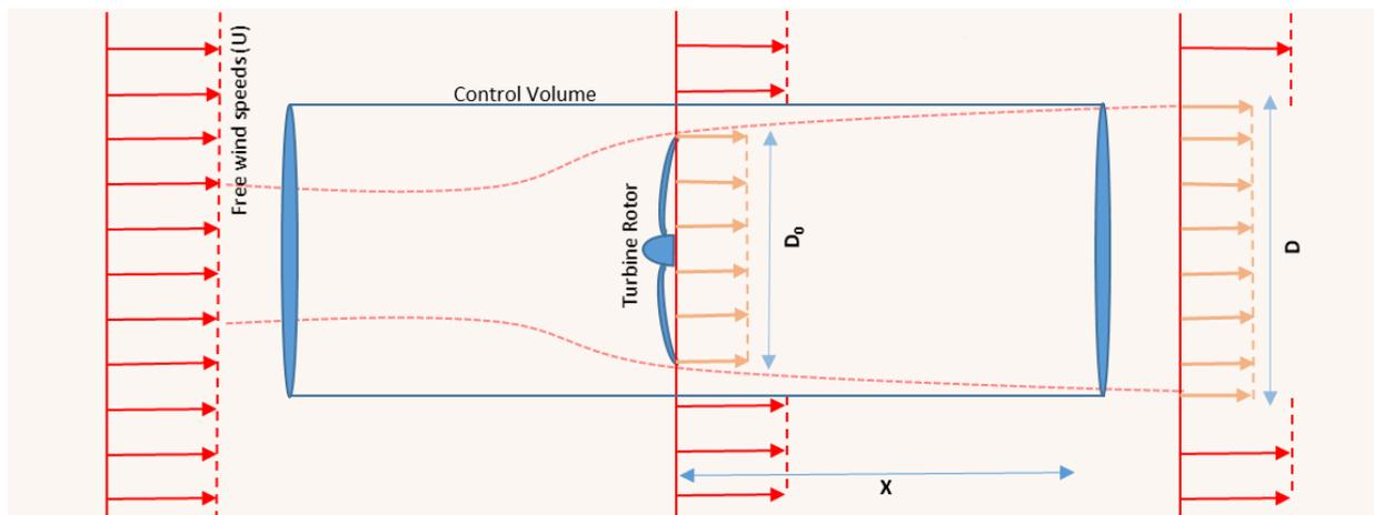
**Figure 3-4: Frandsen wake model using control volume concept**
