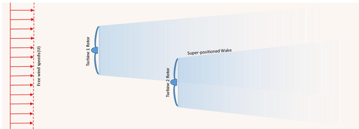
**Figure 3-5: Super-positioned wake between turbines**
