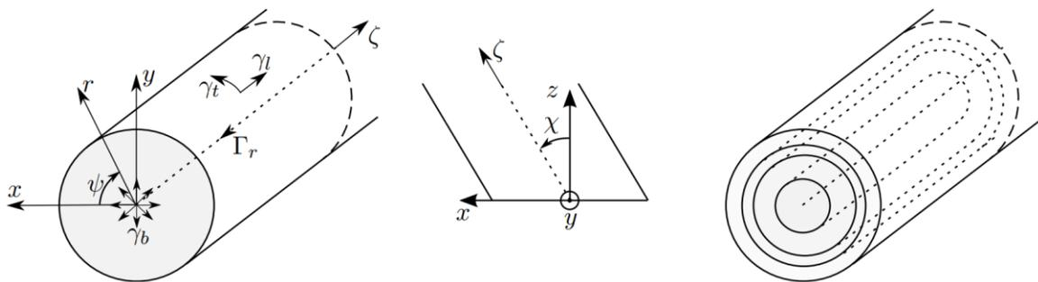
Figure 4-2: Vortex model used by Branlard<sup>19</sup>
