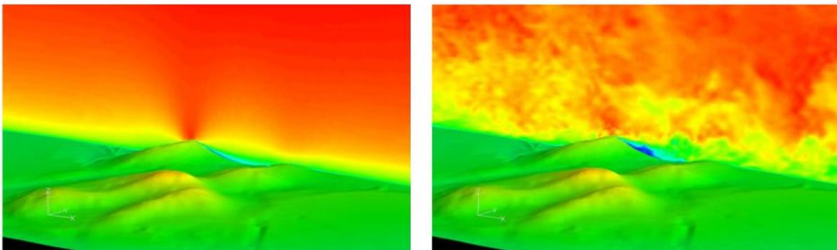
**Figure 2-2: Askevia Hill Flow field (RANS vs LES CFD) Simulations<sup>4</sup>**
