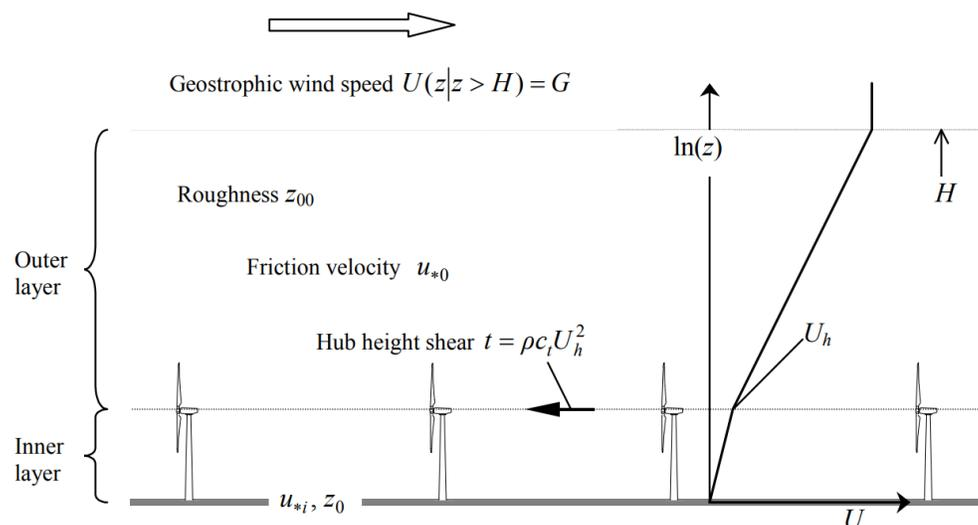
**Figure 3-6: Speed deficit due to infinite array setup**
