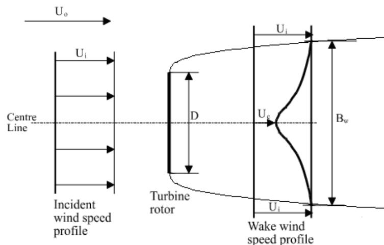
**Figure 3-3: Eddy viscosity wake model as implemented in WindFarmer<sup>11</sup>**
