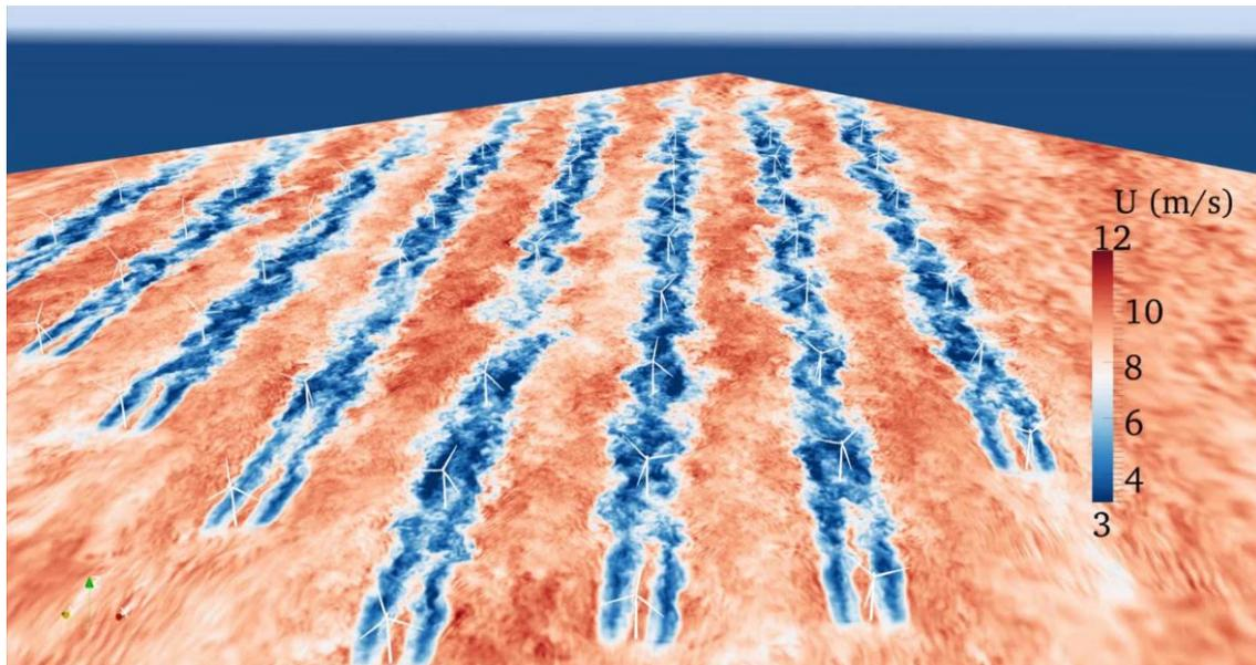
**Figure 2-3: Large-Eddy simulations for wind farm applications<sup>5</sup>**
