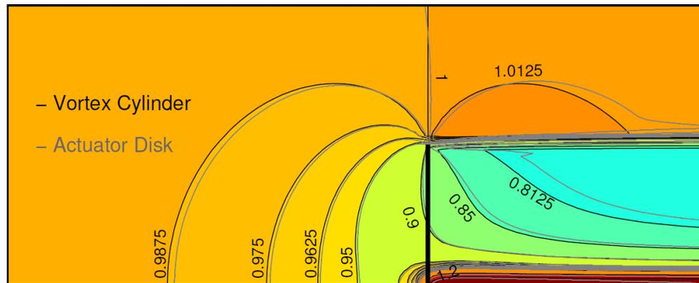
**Figure 4-3: Vortex Cylinder induction effect on an Actuator disk model**
