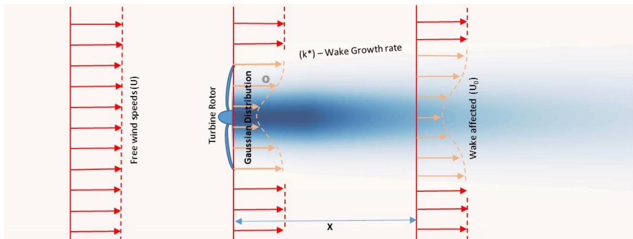
Figure 3-2: Bastankhah- Gaussian wake model<sup>9</sup>
