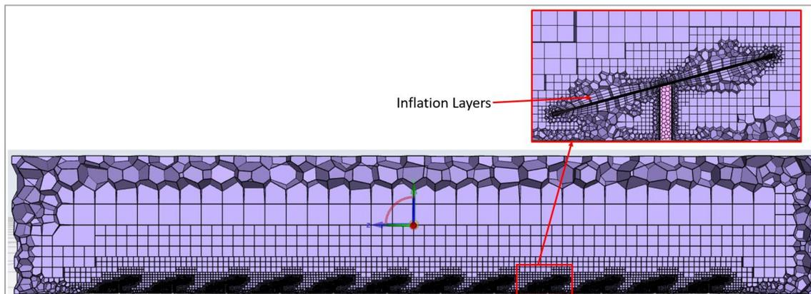
**Figure 5-5: Meshed Model Cross-section**
