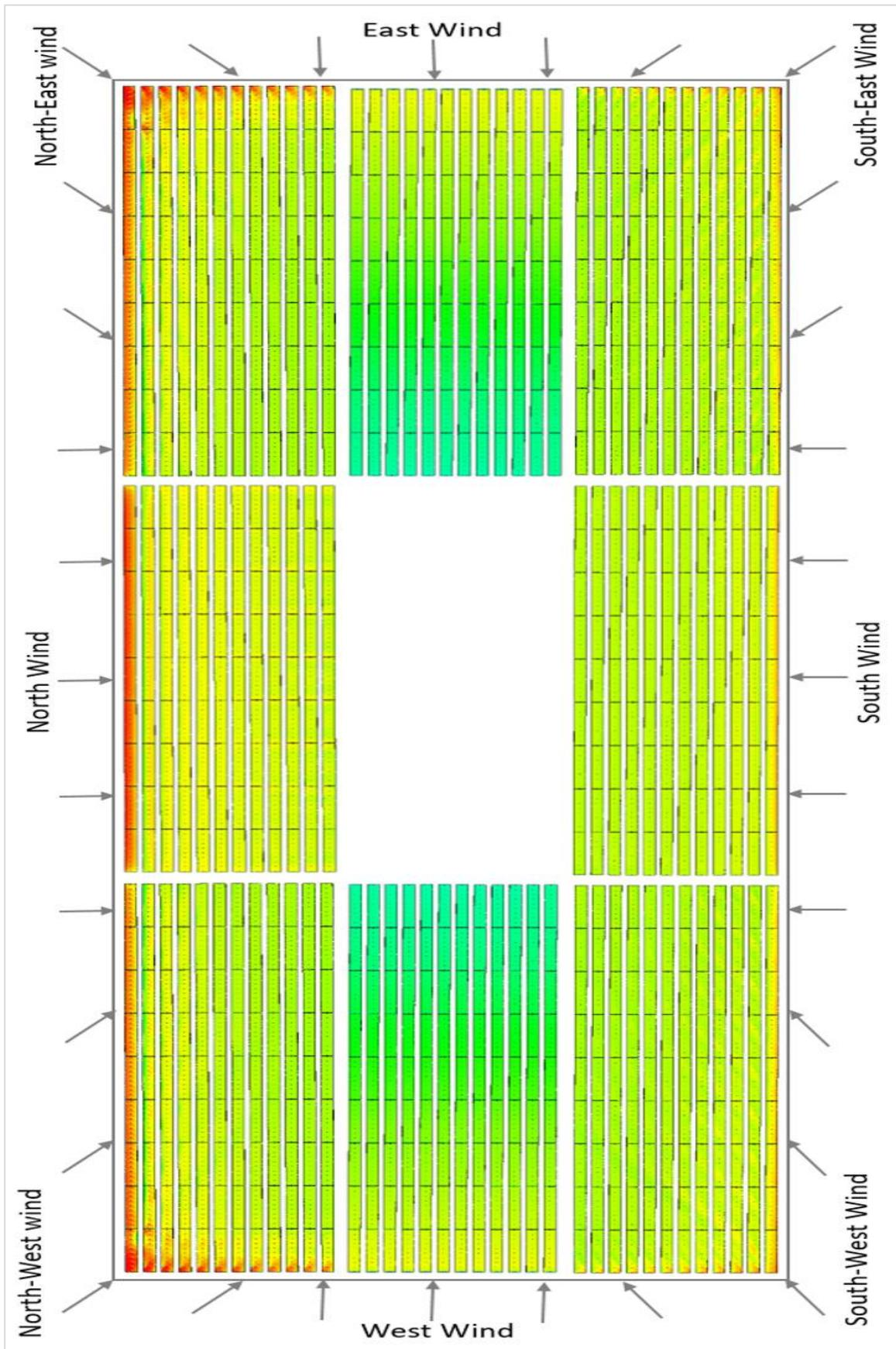
Figure 7-2: Pressure contour for eight wind direction
