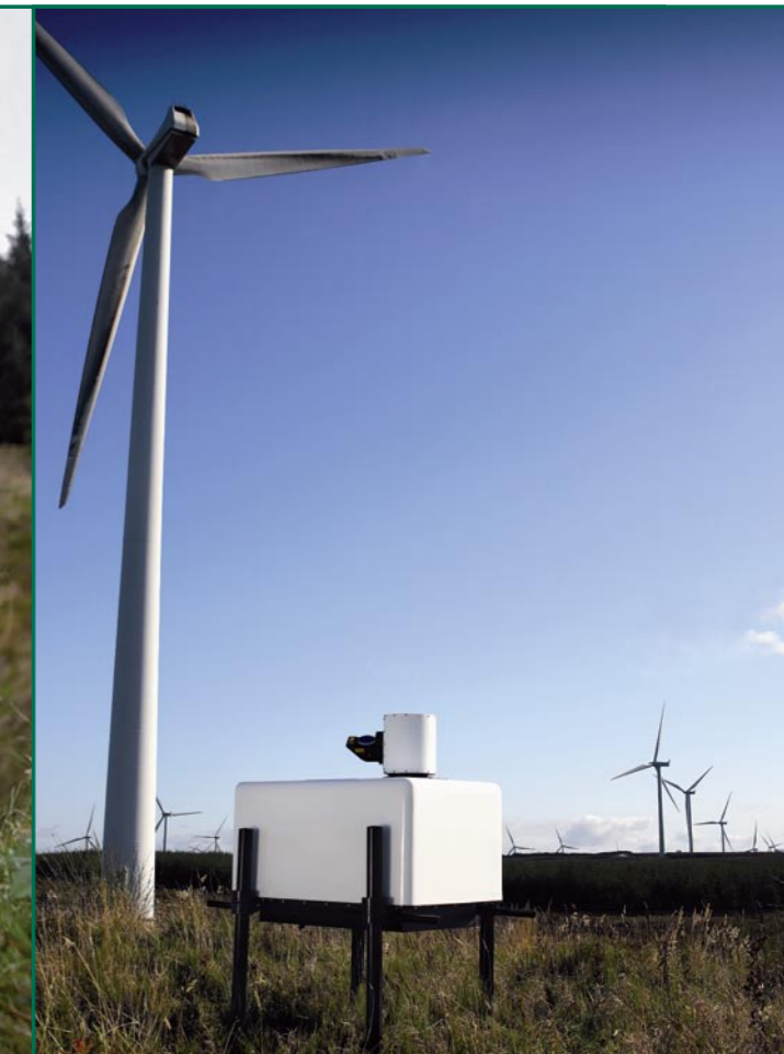
Figure 7. Galion deployed on a wind farm in Scotland
